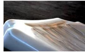
**Uneven moulds:** Do your chairs have a smooth finish? Some chairs are manufactured using poor quality moulds, creating a poor quality finish.
